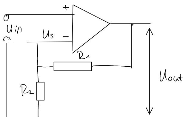
$$U_S = U_{in} - k_r \cdot U_{out} = U_{in} - \frac{R_2}{R_1 + R_2} \cdot U_{out}$$
