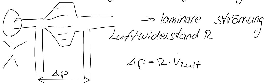
$$\text{"Flow"} = \frac{d \dot{V}_{Luft}}{dt} = \dot{V}_{Luft} \xrightarrow{\dot{V}} k_1 = R \xrightarrow{\Delta P} \Delta P$$
