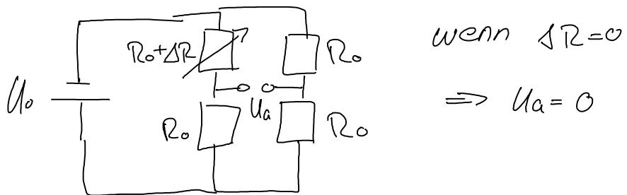
$$U_a = 0, \text{ wenn } \frac{R_1}{R_2} = \frac{R_3}{R_4}$$
